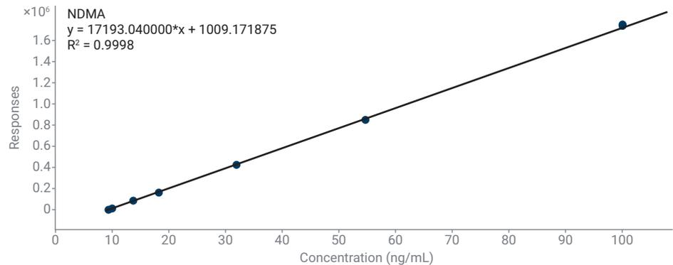
**Figure 4.** Representative calibration curve for NDMA dispersed throughout the chromatogram. The calibration curve fit used a 1/x weighting factor.
