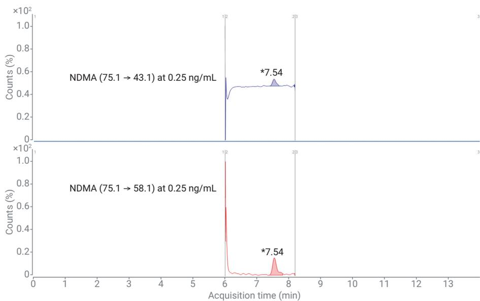
**Figure 3.** Representative extracted ion MRM chromatogram of NDMA (0.25 ng/mL).
