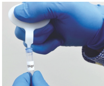
Figure 3 Removing reagent caps Hold the tube in gloved hand, and roll thumb in forward motion over the cap to loosen or, using the decapping tool provided, insert the tooth of the decapper into the inner lip of cap, and gently rotate the tool backwards.
