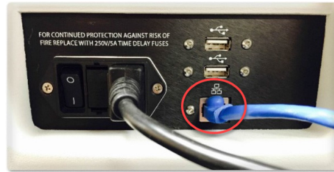
Figure 30. Ethernet port with wired network connection cable
