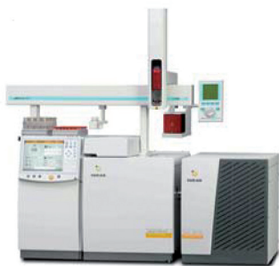
Figure 2. Varian 240-MS Ion Trap mass spectrometer with 450-GC and CombiPAL AutoSampler.
