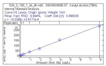
Figure 3. Calibration curve for t-butyl alcohol (TBA) from 0.5 to 40 ppb. Although typically a very poor purge-and-trap compound, it shows excellent response on the 240-MS GC/MS.
