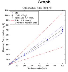
Figure 4a. Calibration curve regression graph for EDB obtained as output from the LCMRL calculator.
