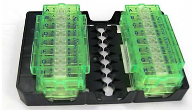
Figure 1 | Seahorse XFp Carrier tray holding 2 cartridges supported by miniplates.
