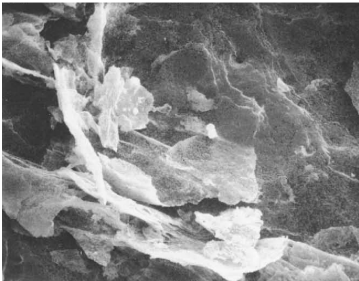
Figure 45a. Scanning electron micrograph (2,000×; palladium deposited with ascorbic acid; graphite heated to 1000 °C)
