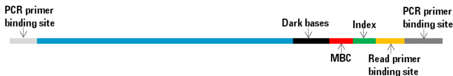
Figure 5 Content of HaloPlex HS-enriched target amplicons. Each amplicon contains one target insert (blue) surrounded by the Ion Torrent sequencing elements (black and yellow), the sample index (green), and the molecular barcode (red).
