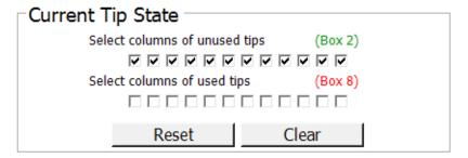
Also verify that the used tip indicator (bottom portion, Box 8) matches the configuration of used tips in the tip box at Bravo Deck position 8.
