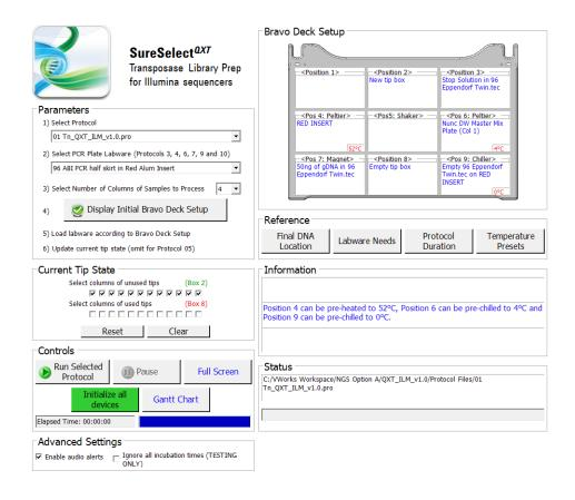
**5** Verify that the **Current Tip State** indicator on the form (shown below) matches the configuration of unused tips in the tip box at Bravo Deck position 2.
