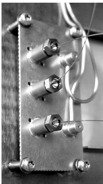
Figure 1. A close-up view of the new micro-fluidic Deans switch in the 6890N GC.
