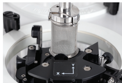
The versatile 280-DS Vessel Module taking basket height (top) and basket wobble (bottom) measurements.
