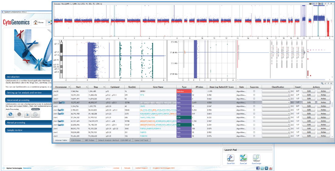
Figure 3. Triage view window in Agilent CytoGenomics Software showing the genome overview, chromosome view of chromosome 17, zoomed-in gene view with interpretation tracks, and aberration table.
