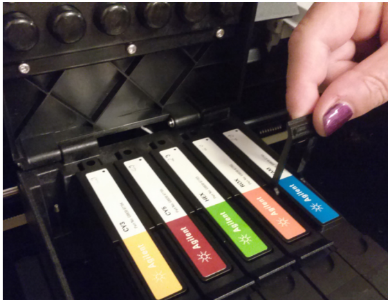
Figure 43 Lifting the hinged tab on an optical module
