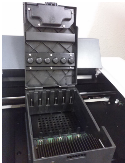
Figure 7 Slots for the optical modules
