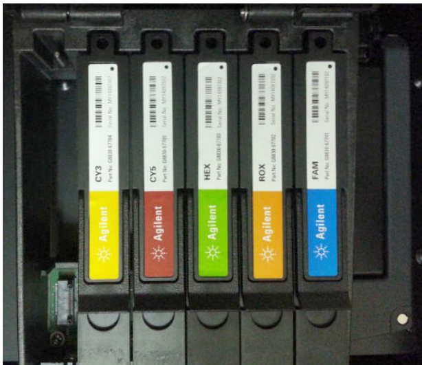
Figure 10 Installed optical modules
