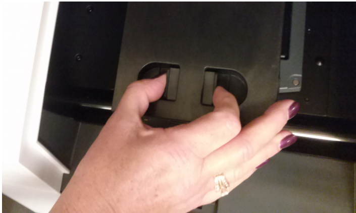
Figure 6 Opening of the optical module housing
