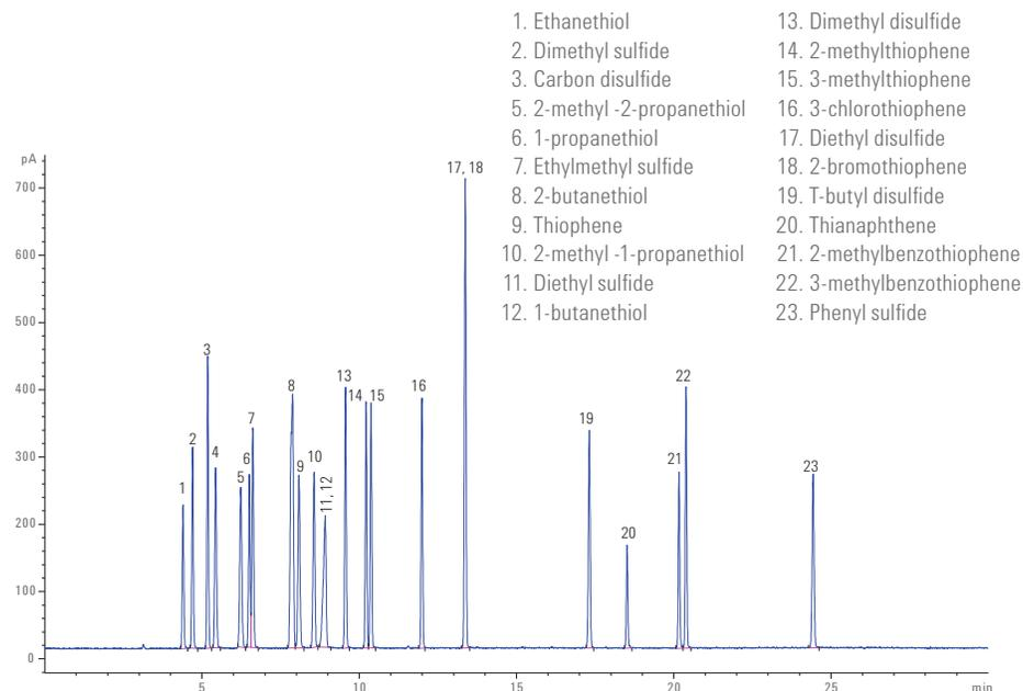
This chromatogram demonstrates performance by showing 23 sulfur standards in isooctane detected at 1 ppm. The Agilent 7890B GC and integral 8355 SCD delivers the ultimate in sulfur analysis with enhanced 'walk-up' readiness. By reimaging the entire analyzer from injection to detection, the Agilent 8355 SCD has set new levels of expectation for sulfur chemiluminescence detectors.
