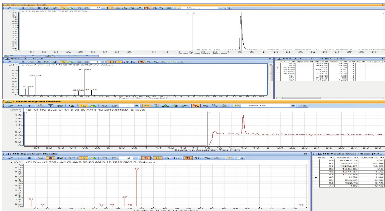
Figure 4. EI and CI chromatogram and spectra of Standard 4, 100% ^{13}\text{C}_7 -Ethanol.
