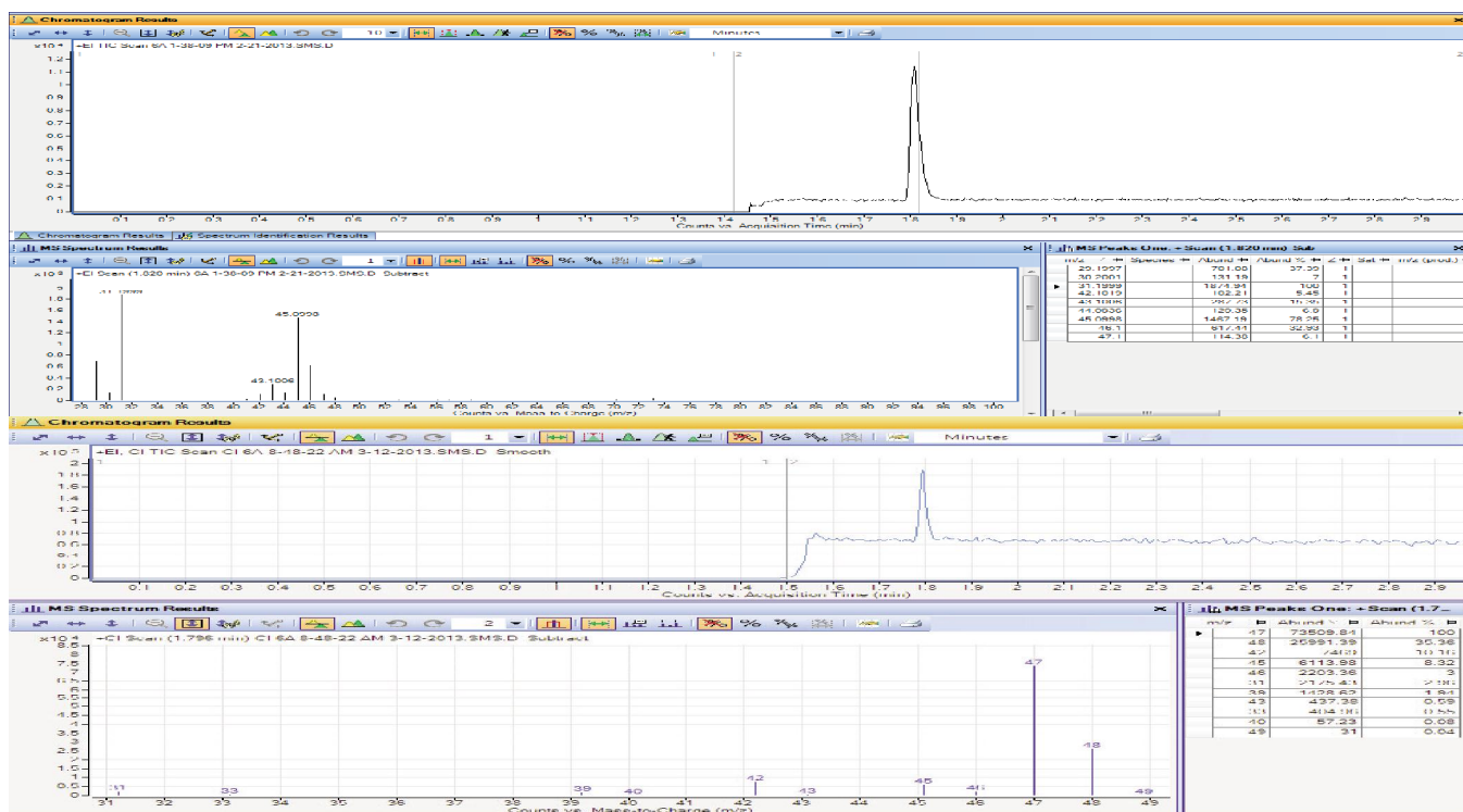
Figure 6. EI and CI chromatogram and spectra of Sample 2, 70:30 ^{12}\text{C} : 2.13\text{C} .
