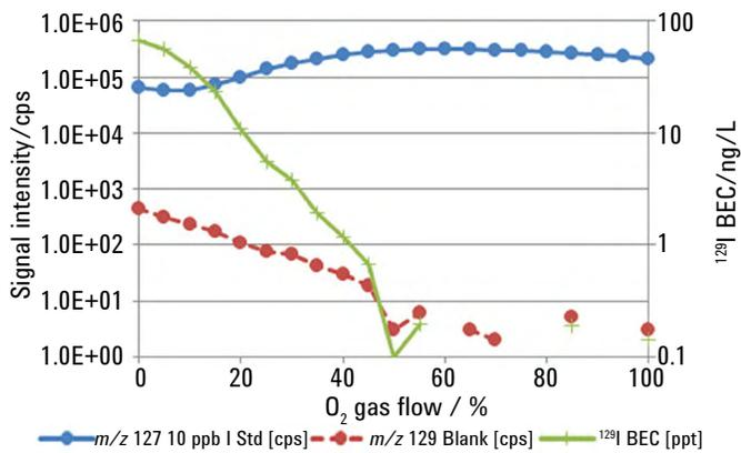
**Figure 1.** Profile of  $^{127}\text{I}^+$ ,  $^{129}\text{Xe}^+$  signals and estimated  $^{129}\text{I}$  BEC. For the BEC calculation, the sensitivity of  $^{129}\text{I}$  was assumed to be the same as  $^{127}\text{I}$ . Scale of  $\text{O}_2$  flow: 100% = 1.12 mL/min.
