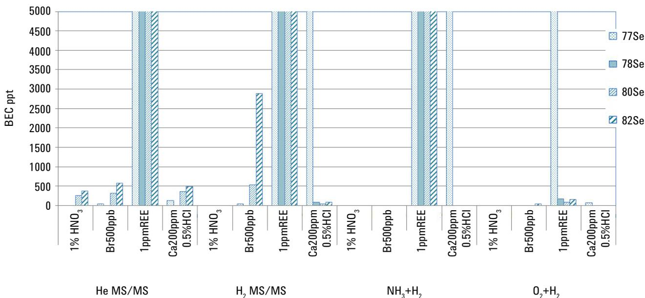
**Figure 1.** Preliminary study of the effectiveness of different cell gases for interference removal. Four synthetic matrices likely to give rise to interferences on the Se isotopes were measured using each of the 4 different cell gas modes.
