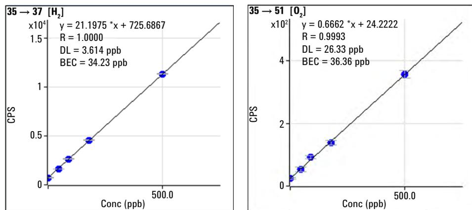
**Figure 3.** Calibration plots for Cl in NMP. Left: H<sub>2</sub> mass-shift method (Q1 = 35, Q2 = 37). Right: O<sub>2</sub> mass-shift method (Q1=35, Q2=51)
