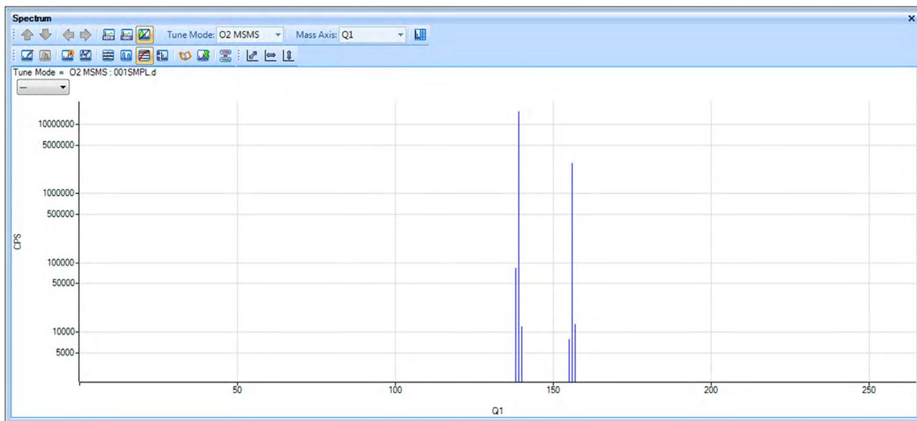
**Figure 3.** Precursor ion scan from 2-260 amu for product ion mass 156, in a 50 ppm La matrix. Six peaks are seen at  $m/z = 138, 139, 140, 155, 156$  and  $157$ , with the intense peaks at  $m/z$  139 and  $m/z$  156 being due to  $^{139}\text{La}^+$  and  $^{139}\text{La}^{16}\text{OH}^+$  respectively.
