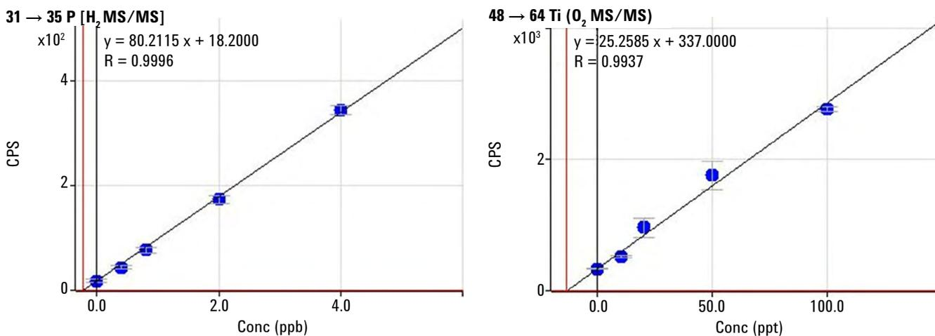
**Figure 1.** MSA curves of P and Ti in 2000 ppm Si
