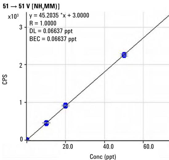
**Figure 2.** Calibration curve of V in 9.8% H<sub>2</sub>SO<sub>4</sub>
