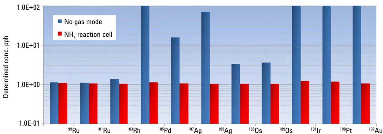
**Figure 1.** Result of synthetic matrix sample test. 1 ppb noble metals were measured in a multi-matrix sample containing 10 ppm of each Cu, Zn, Sr, Rb, Ni, Mo, Pb, Zr, Nb, REEs, Ta, Hf, W and 1 ppm Hg
