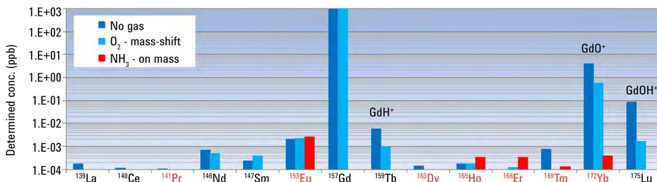
**Figure 1.** Measured concentration of REE impurities in 1 ppm Gd solution. Gd based interferences are observed on Tb, Yb and Lu. Only the elements in red were measured in NH<sub>3</sub> on-mass mode.
