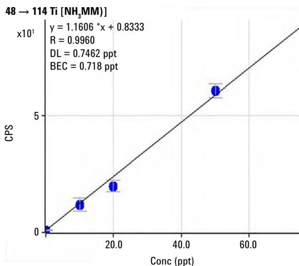
**Figure 1.** Calibration curve of Ti in 9.8% H<sub>2</sub>SO<sub>4</sub>
