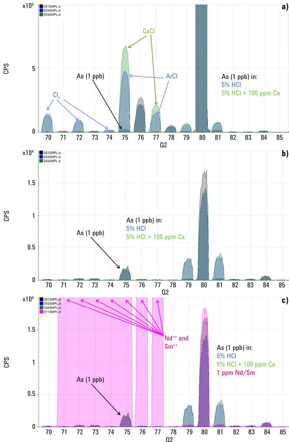
**Figure 1. a)** As<sup>+</sup> (*m/z* 75) in no gas mode, showing polyatomic interferences from ArCl<sup>+</sup> and CaCl<sup>+</sup>; **b)** ArCl<sup>+</sup> and CaCl<sup>+</sup> polyatomics are removed in He collision mode; **c)** He collision mode fails to remove Nd<sup>++</sup> and Sm<sup>++</sup> interferences at *m/z* 75.
