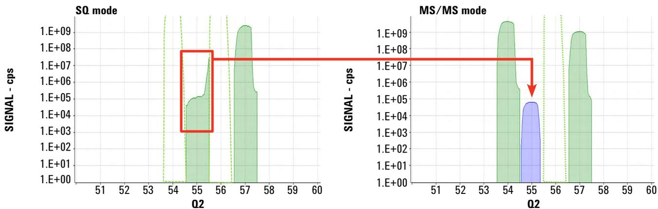
**Figure 1.** Comparison of no gas mode spectra for 500 ppm Fe solution, measured in SQ mode (left) and MS/MS mode (right). The signal colored blue was obtained in pulse counting while the green signal was obtained in analog mode. The dotted lines indicate over-range peaks (automatically skipped to protect the EM detector).
