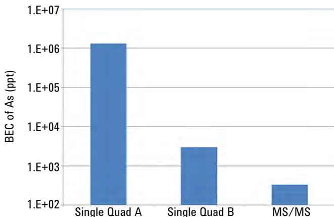
**Figure 1.** BEC of As in 1000 ppm Co solution with O<sub>2</sub> mass-shift method using three acquisition modes (note log intensity scale).
