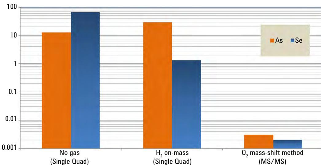
**Figure 2.** BEC of As and Se in 1ppm REE mixed solution with three measurement modes: no gas,  $\text{H}_2$  on-mass and  $\text{O}_2$  mass-shift mode.
