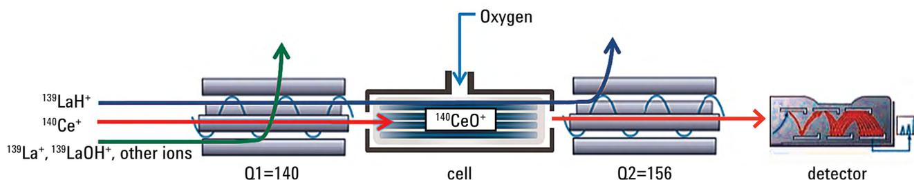
**Figure 1.** MS/MS mass-shift method with  $\text{O}_2$  reaction gas; used for the measurement of Ce, as  $\text{CeO}$  at  $m/z$  156, in a La matrix.
