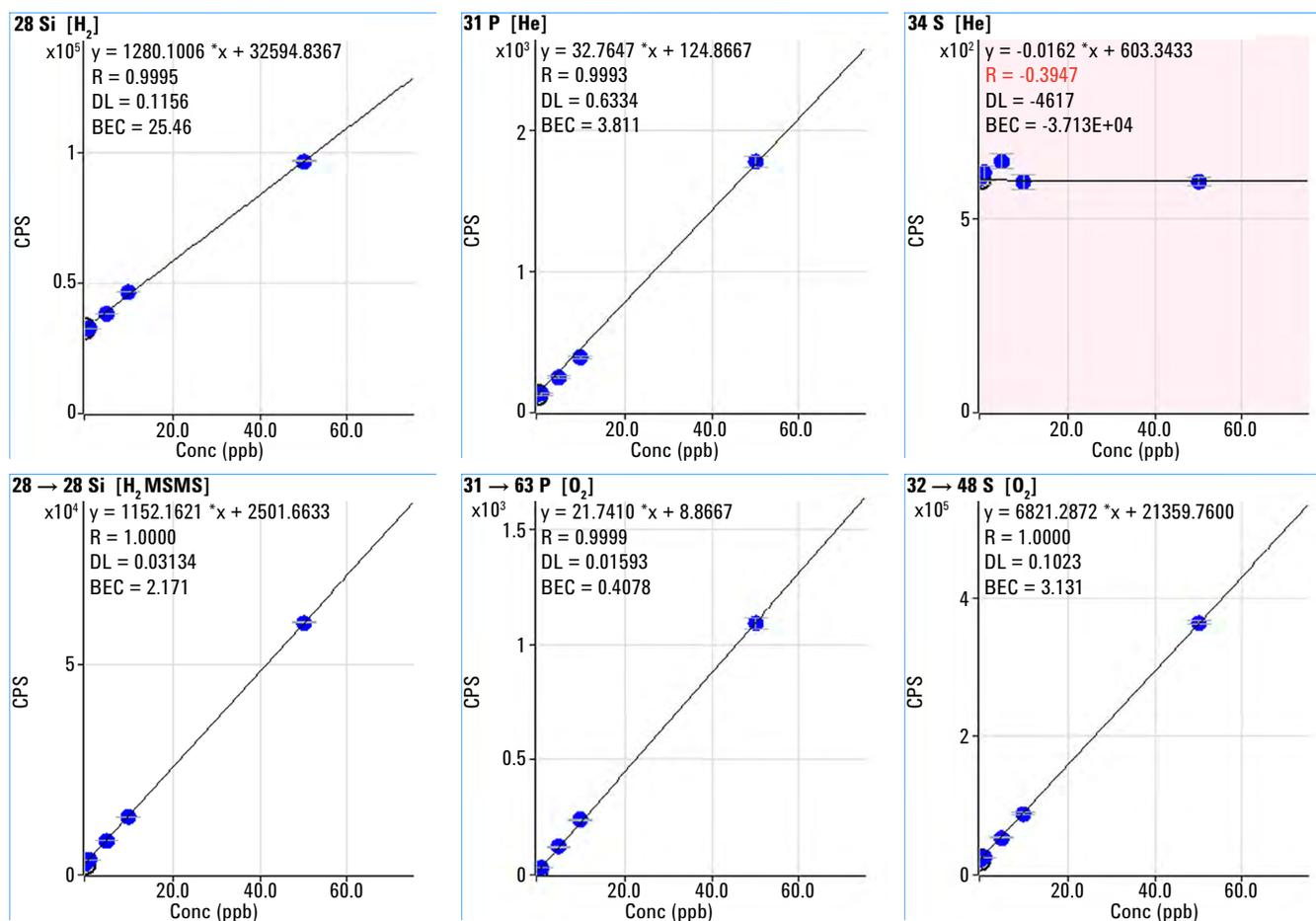
**Figure 1.** Calibration curves for Si, P and S showing SQ results (upper) compared with MS/MS results (lower). <sup>32</sup>S was not measurable at the spiked concentrations in methanol in SQ mode due to the intense <sup>16</sup>O<sub>2</sub><sup>+</sup> polyatomic interference.
