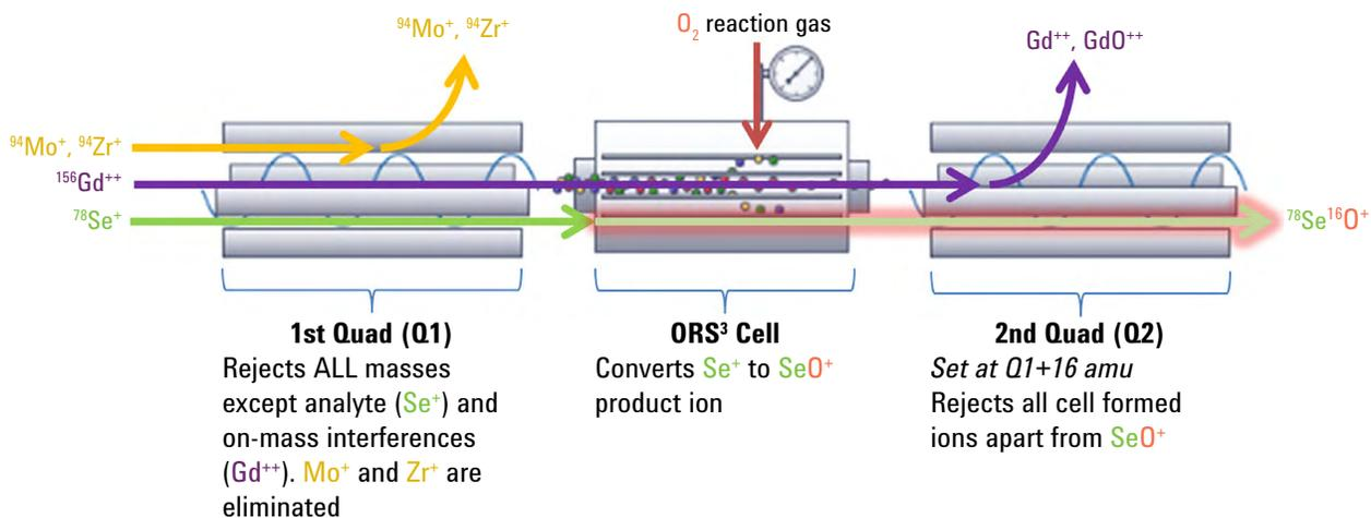
**Figure 1.** Representation of ICP-QQQ setup with Q1 set to 78 amu and Q2 set to 94 amu. Mo and Zr-based interferences are eliminated by Q1 and  $\text{Gd}^{++}$  is eliminated by Q2 allowing the measurement of  $^{78}\text{Se}$  as  $^{78}\text{Se}^{16}\text{O}^+$
