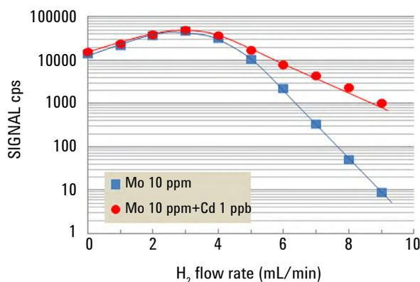
**Figure 1.** (Left): Signal for  $m/z$  111 with 10 ppm Mo and 10 ppm Mo + 1 ppb Cd, plotted as a function of  $\text{H}_2$  flow rate. (Right): Estimated Cd BEC in the presence of 10 ppm Mo as a function of  $\text{H}_2$  flow rate.
