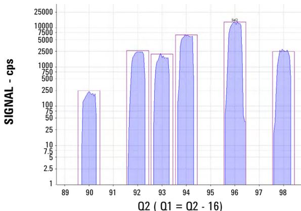
**Figure 2.** Neutral gain scan for 5 ppb Se solution. Note the excellent spectral fit. The six peaks corresponded to  $\text{SeO}^+$  product ions formed from the Se isotopes:  $^{74}\text{Se}$ ,  $^{76}\text{Se}$ ,  $^{77}\text{Se}$ ,  $^{78}\text{Se}$ ,  $^{80}\text{Se}$  and  $^{82}\text{Se}$ .
