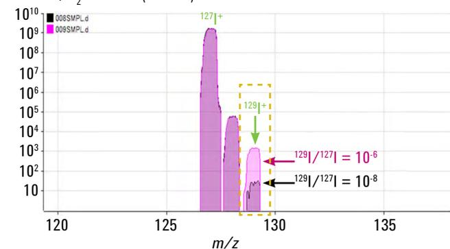
**Figure 2.** Iodine spectra showing both  $^{127}\text{I}$  and  $^{129}\text{I}$  acquired using MS/MS on-mass mode with  $\text{O}_2$  cell gas.  $^{127}\text{IH}^+$  remains to some extent while  $^{127}\text{IH}_2^+$  is completely removed, as noted later.
