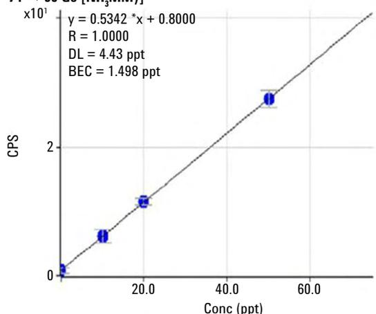
**Figure 1.** Calibration curves of V (NH<sub>3</sub> on-mass mode) and Ge (NH<sub>3</sub> mass-shift mode) in 20% HCl
