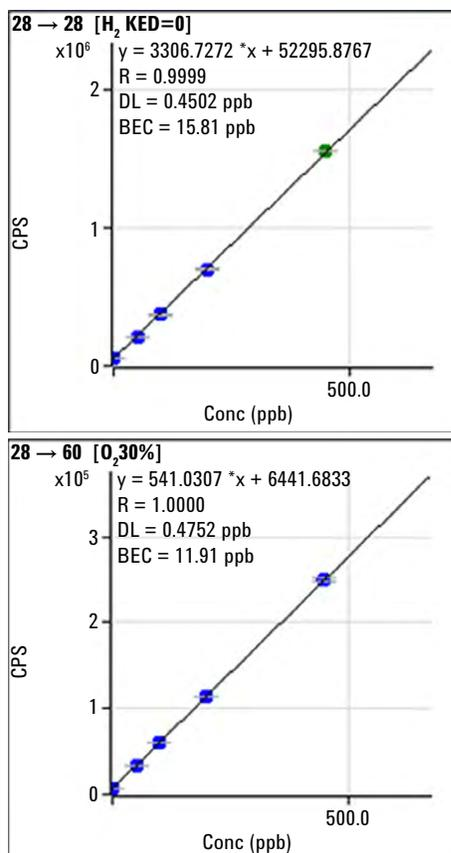
**Figure 2.** Calibration plots for Si in NMP. Top: H<sub>2</sub> on-mass method (Q1=Q2=28). Bottom: O<sub>2</sub> mass-shift method (Q1=28, Q2=60)
