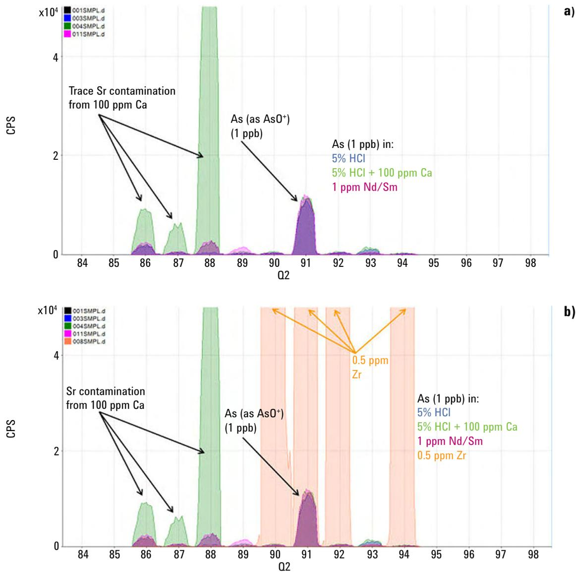
**Figure 2. a)** Nd<sup>++</sup> and Sm<sup>++</sup> interferences at *m/z* 75 are avoided in SQ O<sub>2</sub> reaction mode, by measuring As as the AsO<sup>+</sup> product ion at *m/z* 91; **b)** SQ O<sub>2</sub> reaction mode fails to remove <sup>91</sup>Zr<sup>+</sup> overlap on the AsO<sup>+</sup> product ion.
