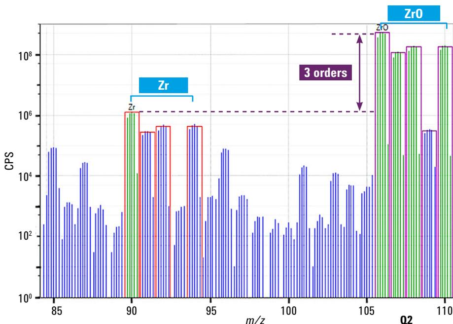
**Figure 2.** Spectrum of 10 ppm Zr obtained using Single Quad mode A with O<sub>2</sub> mass-shift-method
