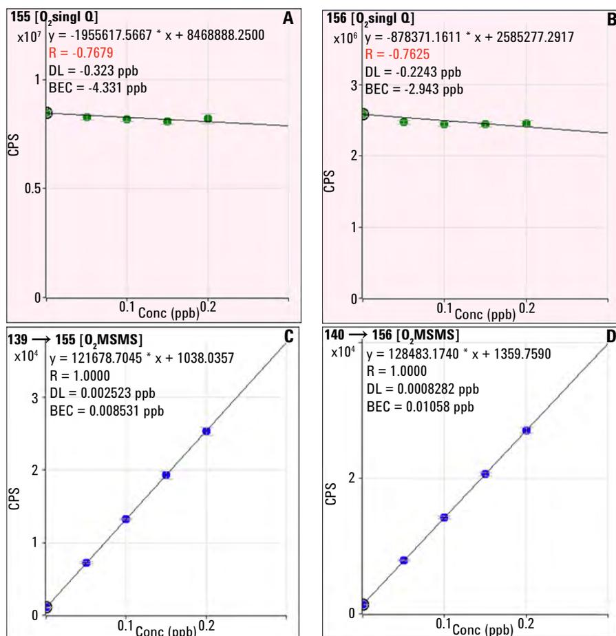
**Figure 2.** Top: Calibration plots up to 0.2 ppb for La in 50 ppm Ba matrix (A) and Ce in 50 ppm La matrix (B), acquired in SQ mode with oxygen reaction gas (emulating conventional quadrupole ICP-MS). Bottom: Calibration plots up to 0.2 ppb for La in 50 ppm Ba matrix (C) and Ce in 50 ppm La matrix (D) acquired in MS/MS mode with oxygen mass-shift.
