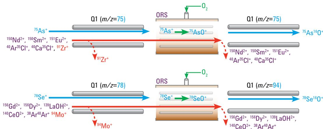
**Figure 1.** ICP-QQQ MS/MS O<sub>2</sub> mass-shift method for measuring <sup>75</sup>As (top) and <sup>78</sup>Se (bottom)
