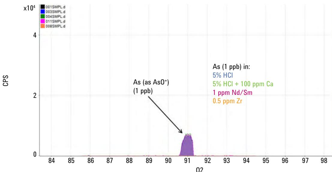
**Figure 3.** MS/MS mass-shift with O<sub>2</sub> reaction mode provides consistent, interference-free measurement of As as AsO in all the matrices.
