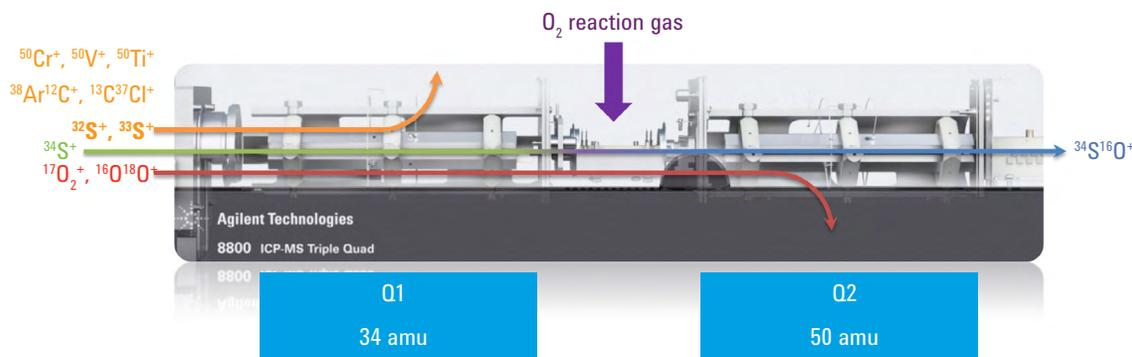
**Figure 1.** Mechanism of MS/MS mass-shift for sulfur isotope analysis. The mass difference between Q1 and Q2 is fixed at 16 amu, so only the  $+^{16}\text{O}$ -atom transition is observed – the other oxygen isotope transitions are eliminated so the original sulfur isotopic pattern is preserved.
