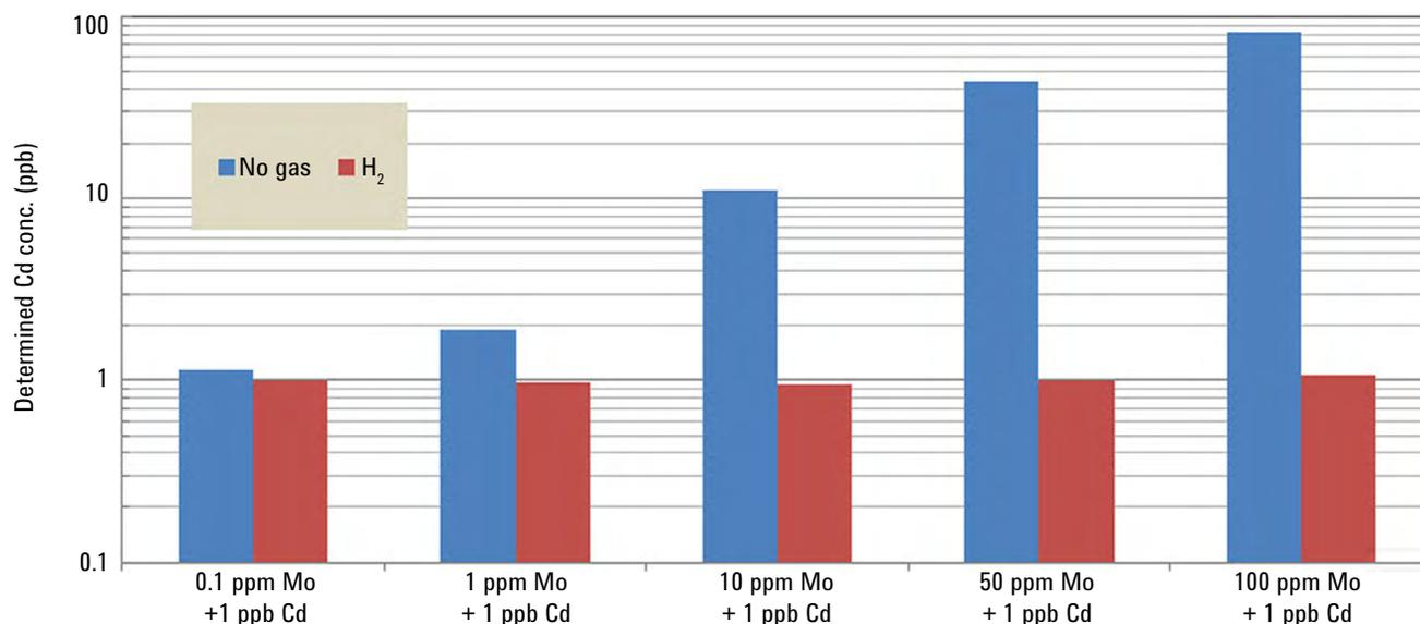
Figure 2. 1 ppb Cd spike recovery in a series of Mo matrix solutions using no gas mode and MS/MS H<sub>2</sub> mode
