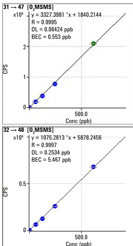
**Figure 1.** Calibration curve using MS/MS with O<sub>2</sub> mass-shift for P (top) and S (bottom) in NMP
