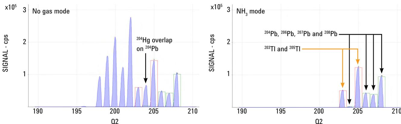
**Figure 1.** Standard solution (1 ppb each of Pb and Tl) spiked with 10 ppb Hg without cell gas (left) and with  $\text{NH}_3$  (right) using MS/MS mode; Note the  $^{204}\text{Hg}$  interference on  $^{204}\text{Pb}$  in no gas mode.
