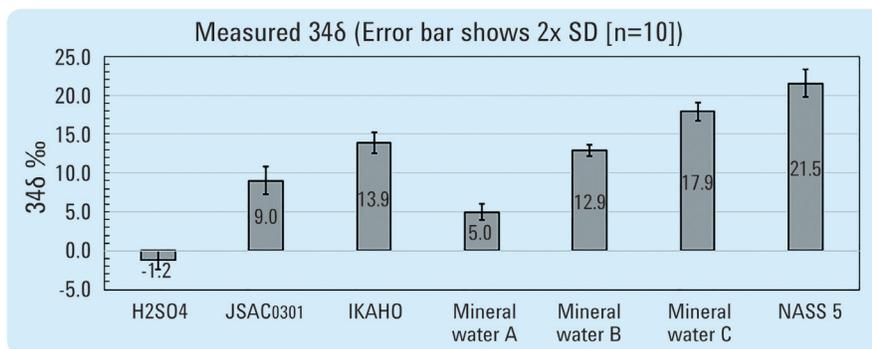
**Figure 2.** Measured sulfur IR for sulfuric acid, river water CRM, spring water, 3 commercial mineral waters (brands A, B and C) and seawater CRM
