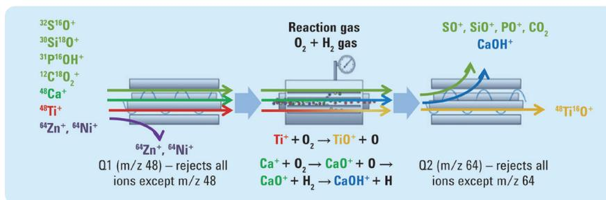
**Figure 1.** Q1 allows only ions at *m/z* 48 to pass to the cell – all other ions are rejected. <sup>48</sup>Ti<sup>+</sup> is converted to <sup>48</sup>Ti<sup>16</sup>O<sup>+</sup> in the cell with O<sub>2</sub>/H<sub>2</sub> reaction gas. Q2 measures TiO<sup>+</sup> at *m/z* 64. <sup>48</sup>Ca<sup>+</sup> reacts to form CaOH<sup>+</sup> at *m/z* 65, so does not interfere with TiO<sup>+</sup> at *m/z* 64
