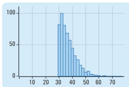
**Figure 2.** Size distribution plot for Anatase reference material
