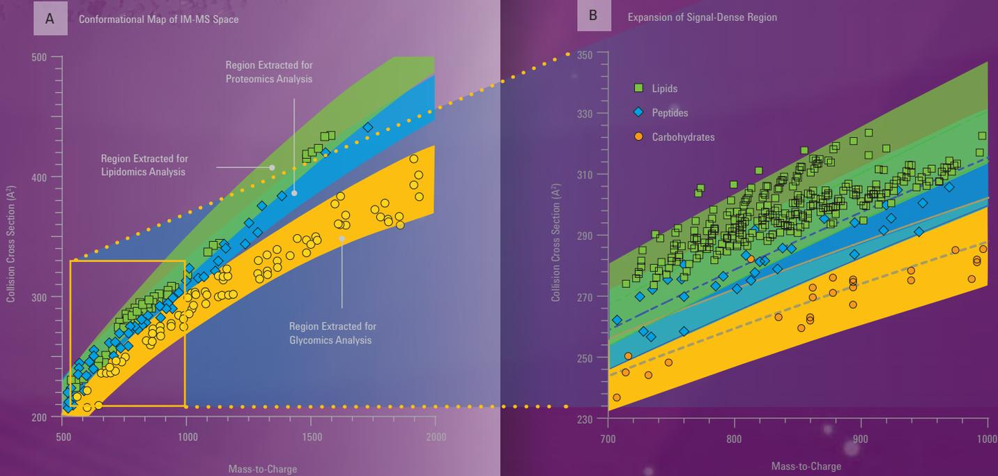
A) Complex sample containing a mixture of lipids, peptides, and carbohydrates was infused directly into the instrument and resolved in 2-D IM Q-TOF analysis by collision cross-section and  $m/z$ . Conformational space maps allow complex mixtures to be separated based on different biomolecular classes, with little front-end sample workup.\*
