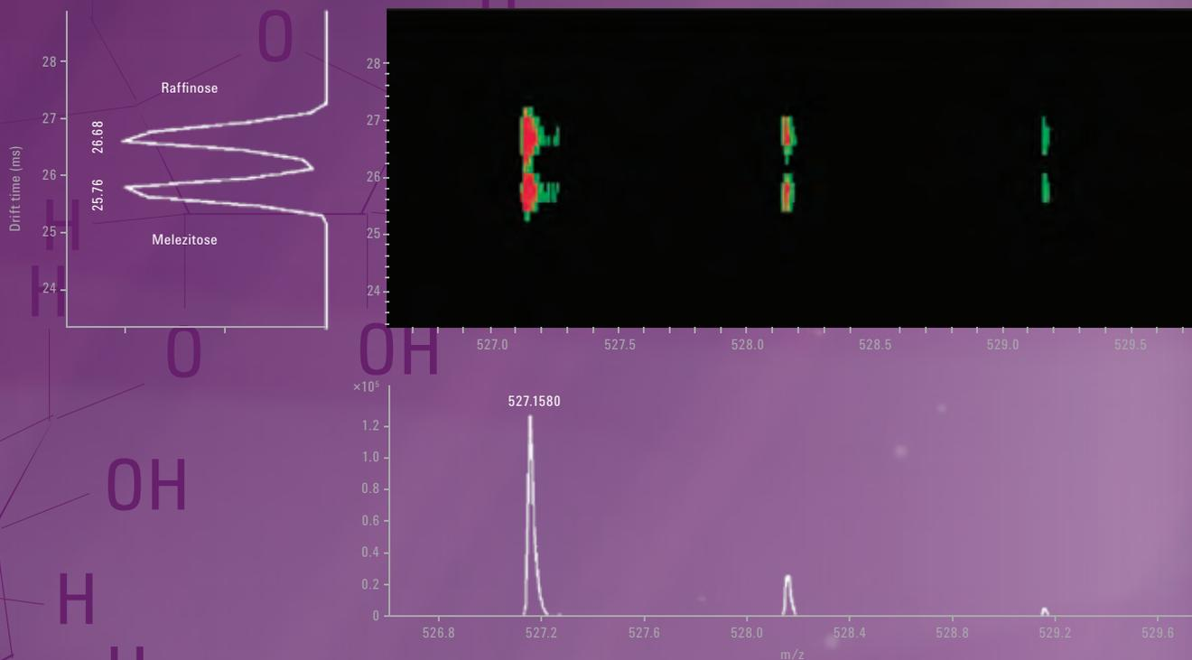
Separation of isobaric trisaccharides using IM Q-TOF: A one-to-one mixture of melezitose and raffinose was infused using a syringe pump. These two carbohydrates can be baseline separated using the ion mobility drift cell and detected using the Q-TOF mass analyzer as sodium adducts. The ion mobility resolving power for this separation is 60.
