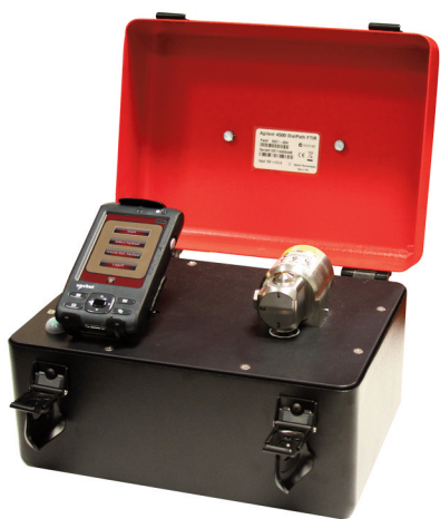
Figure 1. Agilent 4500 Series FTIR with DialPath Technology used for the measurement of FAME in marine diesel and road diesel fuel.
