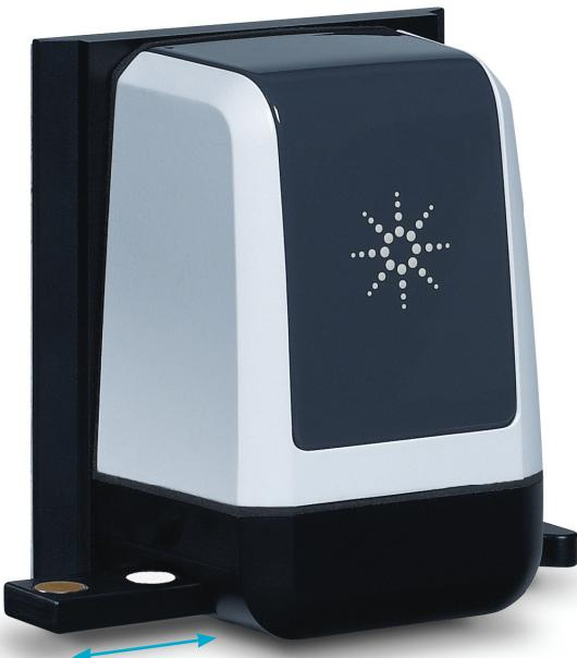
Simply slide the four-position holder to the desired sample position for measurement
