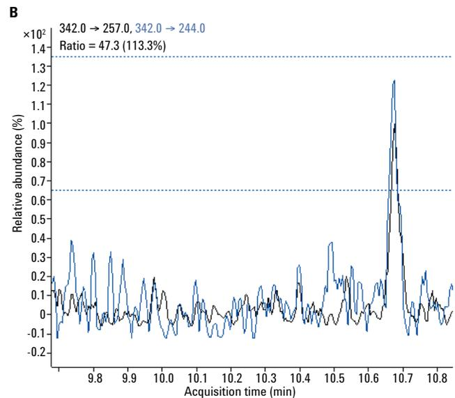
Figure 1. 1.0 ng/mL E1. **A** shows the quantitative SRM 342 → 257. **B** shows the qualitative transition 342 → 244. The dotted lines in **B** represent the allowable uncertainty for qualifier ratio. Noise region for S/N calculation is 10.4 to 10.6 minutes.
