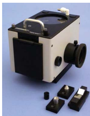
Figure 2. Praying Mantis accessory with alignment tools and powder cell sample cups
