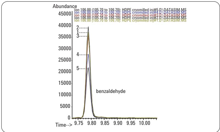
**Figure 7** Multiple headspace extraction data for the benzaldehyde peak from HDPE. The numbers next to the peak indicate the extraction number.
