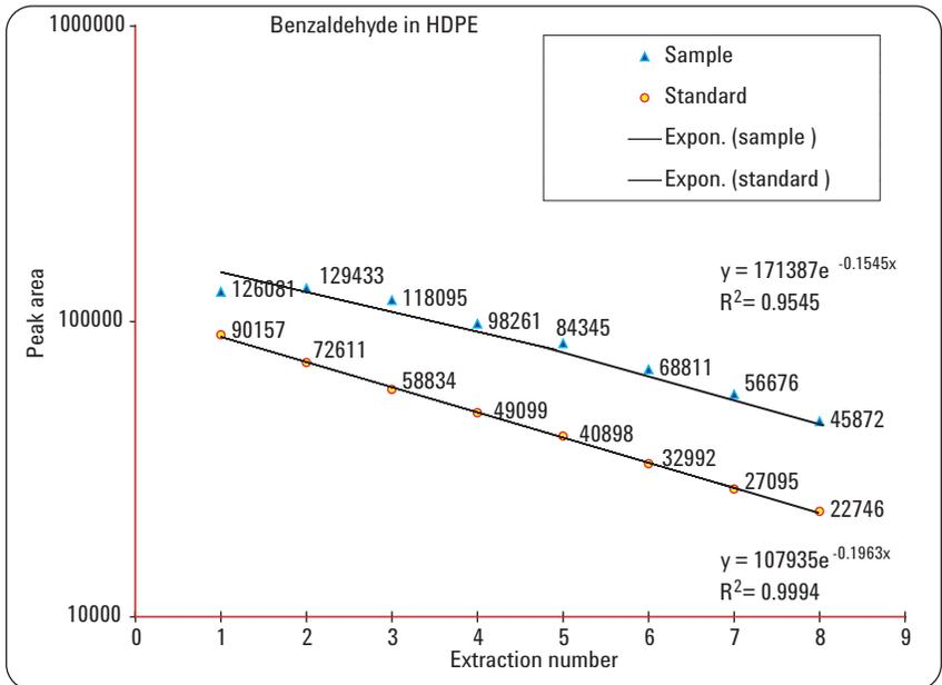
**Figure 8** Semi-logarithmic plot of the MHE raw data for benzaldehyde in HDPE.
