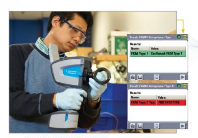
In the MicroLab method chosen for the pictured O-ring analysis, a threshold was set such that samples within the target group are shown in green while those outside the target group are shown in red. Furthermore, the conditional reporting feature can be used to display a customized alert message such as, "Confirmed FKM Type 1" for samples within the target group and the message "NOT FKM TYPE 1" for samples outside the target group.
