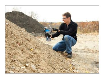
**Control at your fingertips:** An integrated touch screen operates all system and data acquisition functions and tilts for easy viewing in ambient light.
