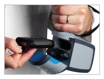
**Longer periods of continuous operation:** The lithium ion batteries that power the 4300 can easily be swapped while the system is running.
