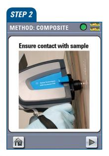
MicroLab Mobile Software will instruct when to position the spectrometer's sample interface on the object to be analyzed.
