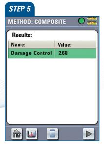
Results screen: The results screen will display the calculated component values relative to their critical limits. Components within the acceptable range are shown in green.
