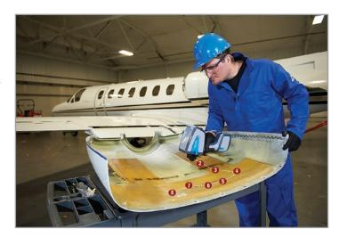
**Real-time measurements:** Agilent MicroLab Mobile Measurement software was created and enhanced for our portable and handheld spectrometers. Its real-time spectral display complements the rapid scanning capability of the 4300 MCT system.
