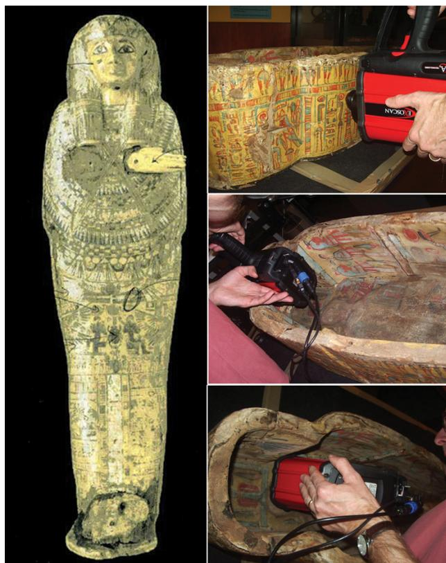
**Figure 14.** Compact size and ideal sampling interface configuration allow Agilent handheld FTIR systems to investigate curved, less accessible areas of this Egyptian sarcophagus Image courtesy of Glasgow Museum
