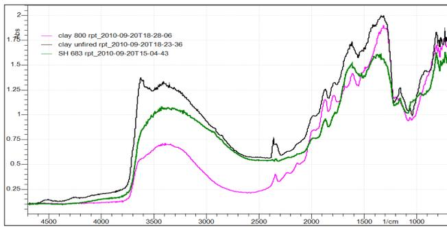
**Figure 11.** The infrared spectra of Orkney Island unfired clay and clay fired at 800 °C are compared to that of a clay fragment found at the site. The latter spectrum indicates that the pottery was fired at between 400 and 600 °C.
