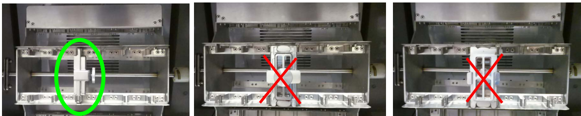
Figure 14 Assembled chambers in correct (left) and incorrect (middle and right) orientations
