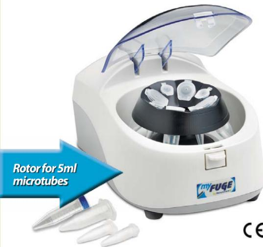
Rotor for 5ml microtubes
