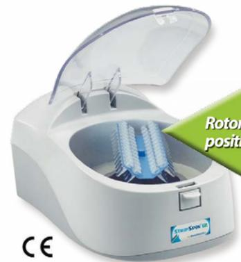
Rotor holds 12 position PCR strips
