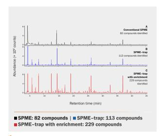
Analysis of tea sample using a variety of SPME approaches, demonstrating how use of a focusing trap increases the number of compounds detected. Multi-step enrichment results in detection of 147 extra compounds over traditional SPME.
