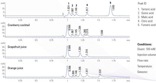
Eluent: 100 mM Potassium phosphate buffer, pH 2.5 Injection volume: 5 µL 0.5 mL/min Flow rate: 50 °C Temperature: Detector: DAD, at 226 nm
