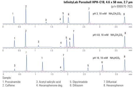
A robust method development process is critical to ensuring that your method is long lasting, stable, and reliable. Because the retention and selectivity of ionizable compounds (such as acids and bases) can change significantly with varying pH, it is becoming standard practice to employ low, medium, and high-pH analyses during method development.
