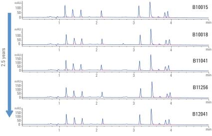
InfinityLab Poroshell 120 EC-C18, 3.0 x 100 mm, 2.7 µm (p/n 695975-902) from five different lots
