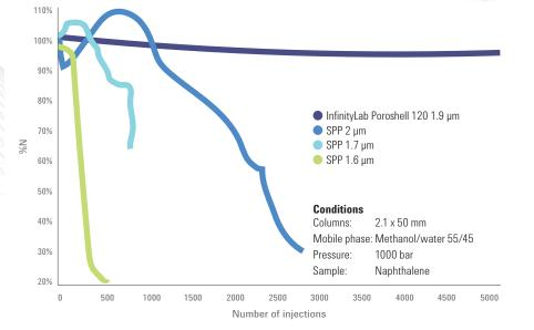
The InfinityLab Poroshell 120 columns showed stability for 5,000 injections under high-pressure UHPLC conditions.
