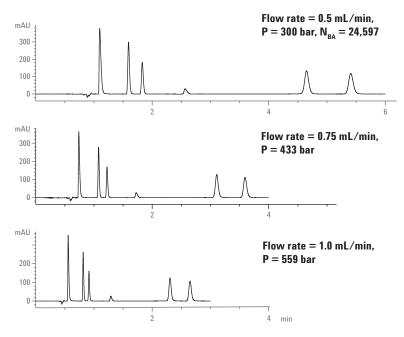
More viscous solvents like methanol can be used at HPLC or UHPLC pressures.
