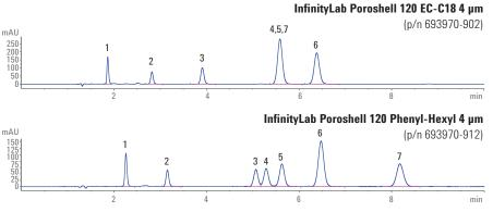
**Choose the phase that takes advantage of key analyte interactions.** Phenyl-Hexyl provides alternative selectivity to EC-C18 for compounds containing phenyl groups. The different selectivity is due to pi-pi interactions with the analytes, as shown in this steroid separation.
