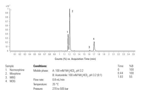
1290 Infinity II LC and 6410 Triple Quadrupole LC/MS
