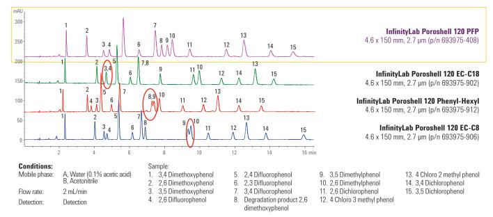
PFP is a pentafluorophenyl ligand, which provides an orthogonal separation mechanism with C18 chemistries. PFP phases can separate analytes based on small differences in structure, substitution, and steric access to polar moieties. The resulting selectivity for positional isomers, halogenated compounds, and polar analytes is particularly useful when analyzing complex mixtures.
