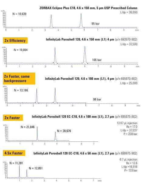
InfinityLab Poroshell 120 is an excellent choice for faster methods at HPLC pressures.
