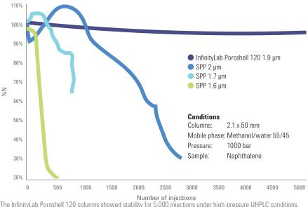
The InfinityLab Poroshell 120 columns showed stability for 5,000 injections under high-pressure UHPLC conditions.
