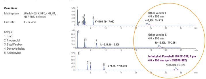
InfinityLab Poroshell 120 columns outperform other columns for challenging analytes.
