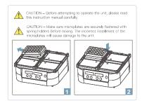
Note: When using deep hole plate, the instrument speed should not exceed 1000rpm.
