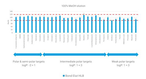
**Figure 1.** Bond Elut HLB demonstrates good recovery for a panel of targets from polar to non-polar targets with MeOH elution. For some non-polar targets, stronger solvents such as 1:1 MeOH/ACN, ACN, acetone, and ethyl acetate can be useful to improve the recovery.
