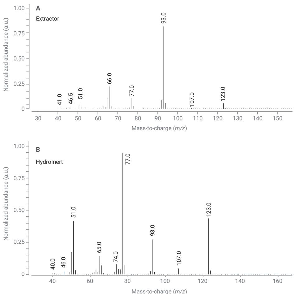
**Figure 2.** Mass spectra for peak eluting at nitrobenzene retention time with hydrogen carrier gas in (A) extractor source with 3 mm extraction lens showing hydrogenation to aniline with the abundant 93 *m/z* ion and (B) Agilent Hydrolnert source, showing an improved mass spectrum that correlates to nitrobenzene.
