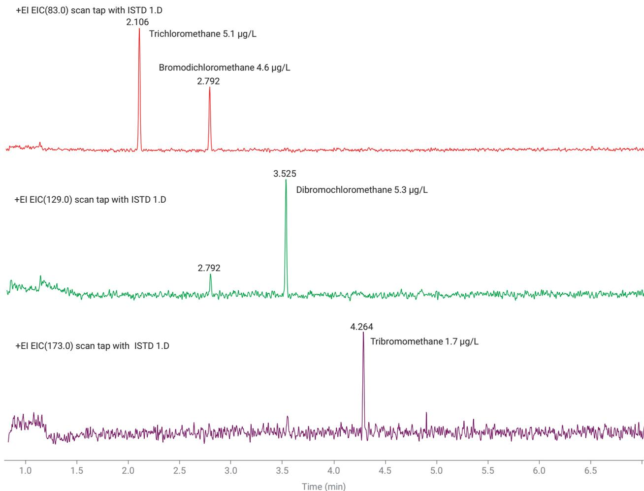
**Figure 14.** Extracted ion chromatograms (EICs) of 83, 129, and 173  $m/z$  with identification and quantification of four trihalomethanes when running a headspace HS/GC/MS system with  $\text{H}_2$  carrier gas and the Agilent HydroInert source.
