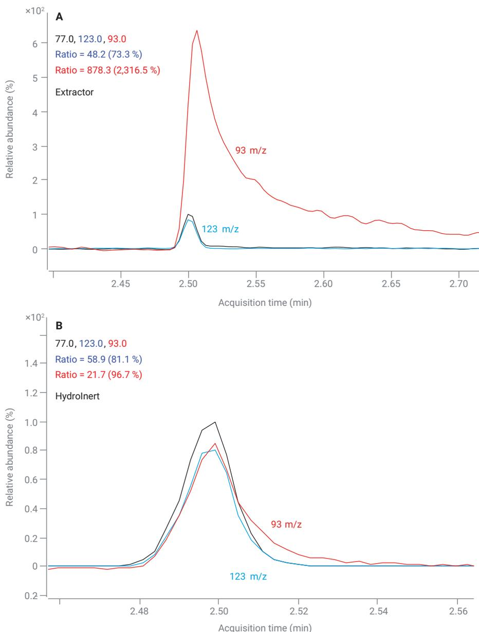
**Figure 3.** EICs of nitrobenzene with hydrogen carrier gas in (A) extractor source with 3 mm extraction lens, showing hydrogenation to aniline with the abundant 93 m/z ion and (B) Agilent Hydrolnert source, showing an improved 123 versus 93 m/z ratio.
