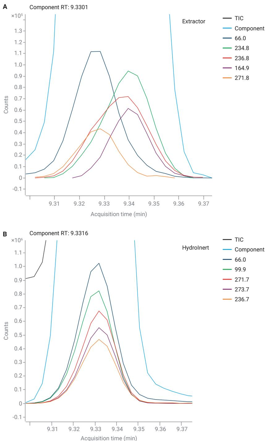
**Figure 5.** EICs of the top five abundant ions for heptachlor with H<sub>2</sub> carrier gas and (A) extractor source with 3 mm extraction lens and (B) Agilent Hydrolnert source with 9 mm extraction lens.
