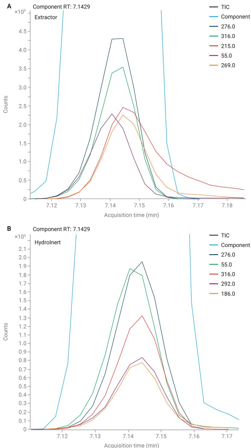
**Figure 12.** EICs of the top five abundant ions for ethalfuralin with H<sub>2</sub> carrier gas and (A) extractor source with 3 mm extraction lens and (B) Agilent HydroInert source with 9 mm extraction lens.
