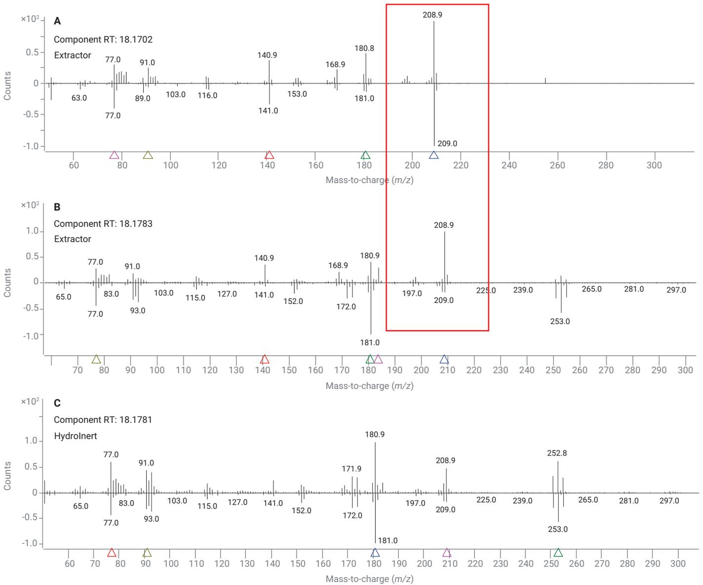
**Figure 13.** Head-to-tail comparison of deconvoluted mass spectrum (top of each subfigure) to library mass spectrum, NIST17.L (bottom of each subfigure) for deltamethrin with H<sub>2</sub> carrier gas and (A) extractor source with 3 mm extraction lens run 1, (B) extractor source with 3 mm extraction lens run 2, and (C) Agilent Hydrolnert source with 9 mm extraction lens.
