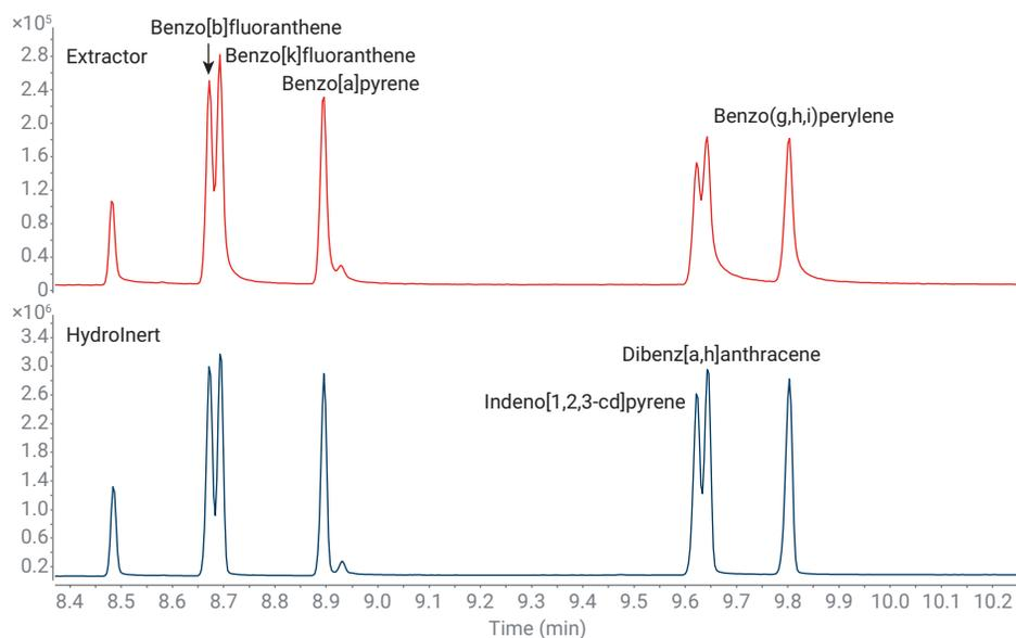
**Figure 11.** Zoom in of later-eluting PAH region to compare peak shape and resolution of these compounds when using H<sub>2</sub> carrier gas with an extractor source and Agilent Hydrolnert source at 50 ng/μL.
