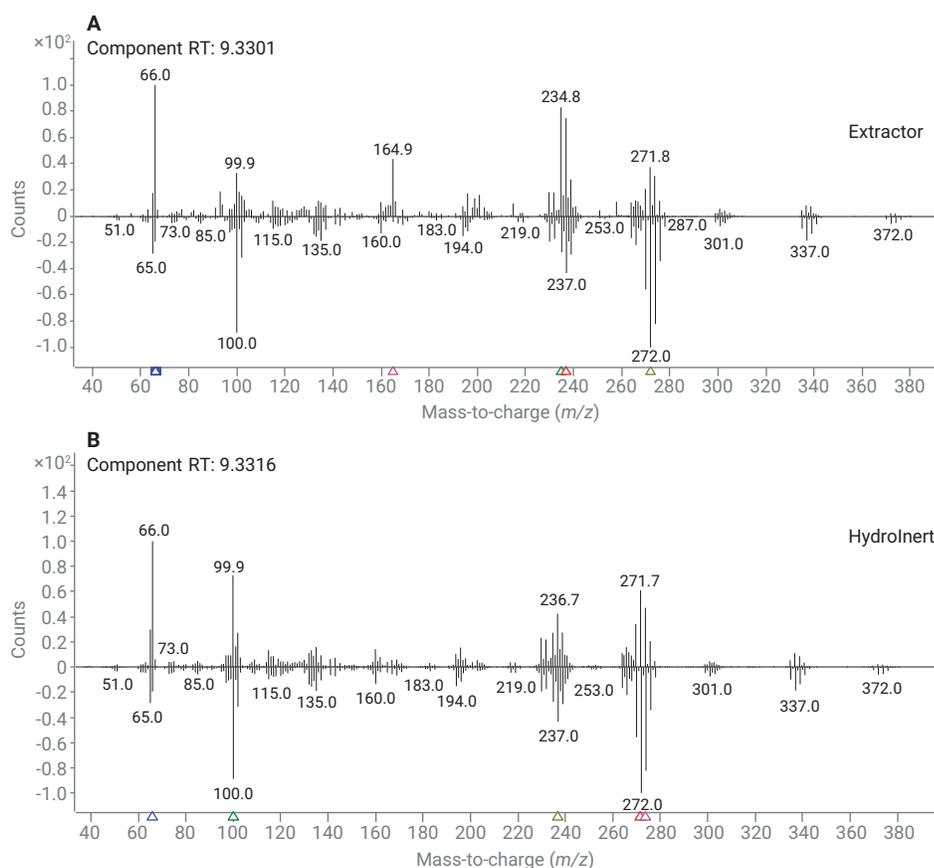
**Figure 4.** Head-to-tail comparison of deconvoluted mass spectrum (top) to library mass spectrum, NIST17.L (bottom) for heptachlor with H<sub>2</sub> carrier gas and (A) extractor source with 3 mm extraction lens and (B) Agilent Hydrolnert source with 9 mm extraction lens.
