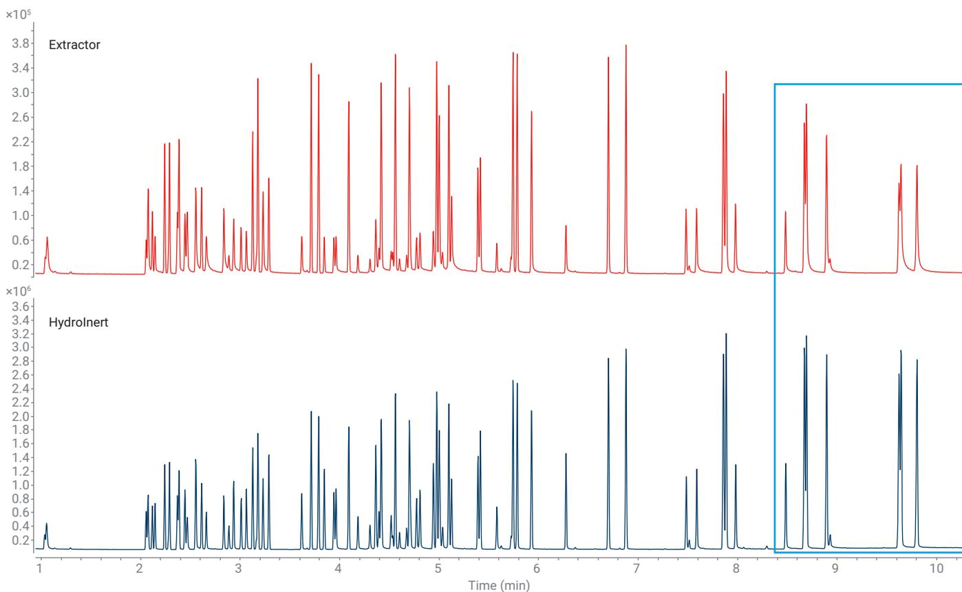
**Figure 10.** Comparison of peak shape and resolution for H<sub>2</sub> carrier gas with an extractor source and Agilent Hydrolnert source for a set of 68 target analytes for EPA method 8270 at 50 ng/μL.
