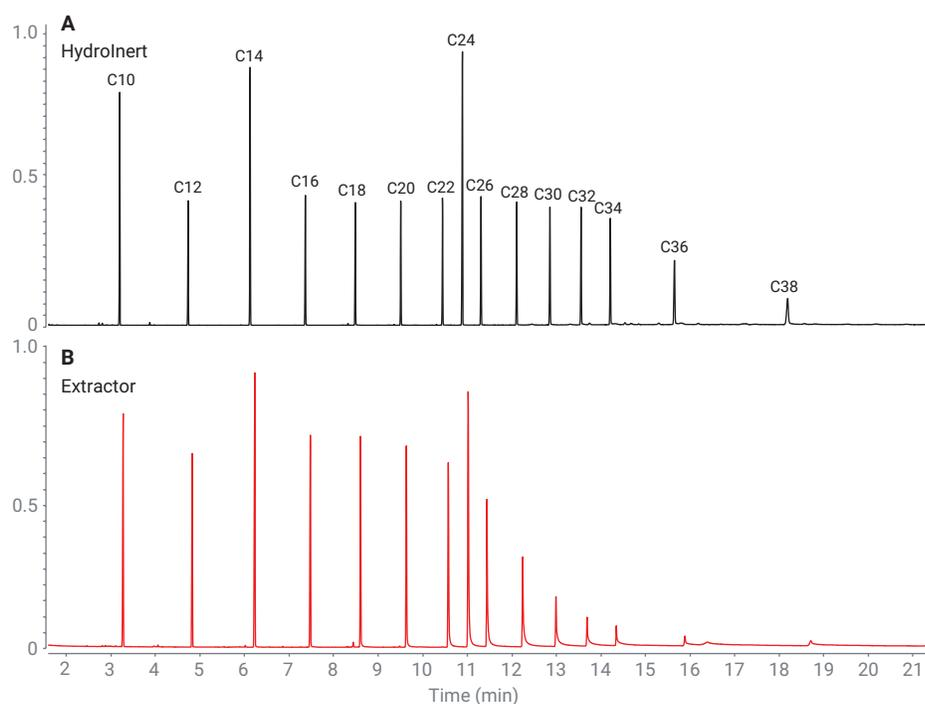
**Figure 8.** TICs of straight-chain hydrocarbons from *n*-decane (C<sub>10</sub>) to *n*-octatriacontane (C<sub>38</sub>) to visually represent the observed tailing (or lack thereof) when using hydrogen carrier gas with the (A) Agilent Hydrolnert source and (B) existing extractor source.
