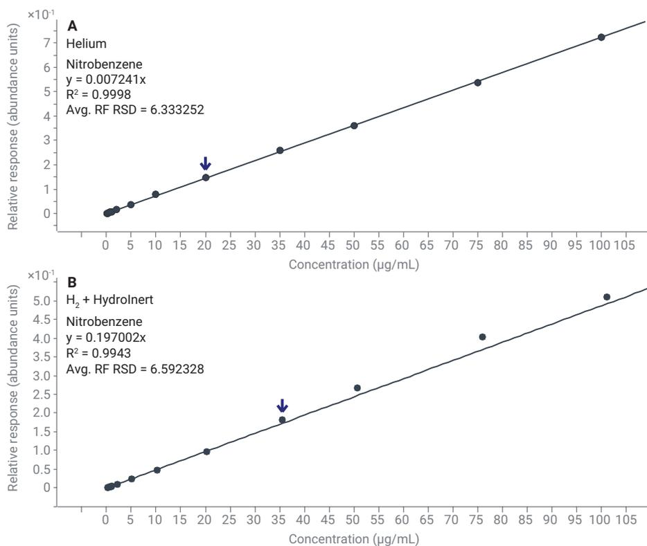
**Figure 9.** Nitrobenzene linear range (0.1 to 100 ng/µL) collected on a GC/MS system in (A) He and (B) H<sub>2</sub> carrier gas, with Agilent HydroInert source.
