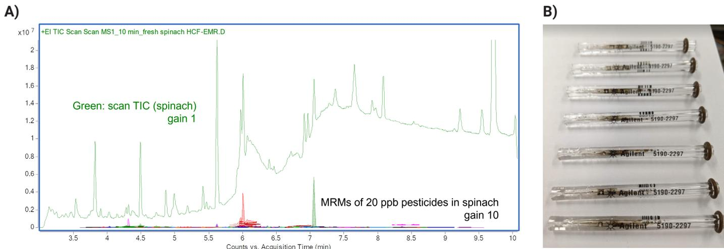
**Figure 8.** (A) TIC of a full scan chromatogram acquired for spinach extract and the MRM TIC for 20 ppb pesticides. (B) The GC inlet liners replaced after 100 injections when analyzing spinach extract during the robustness evaluation.
