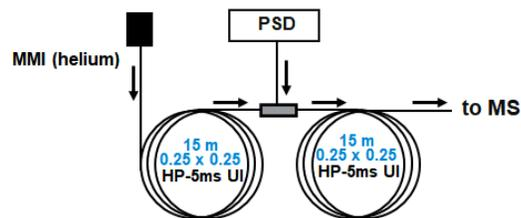
Narrow bore 10 x 10 m midcolumn backflush configuration:
