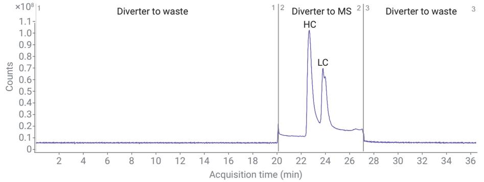
**Figure 3.** Online reduction of Trastuzumab by 2D-LC/MS showing the TIC of SEC in the second dimension separating the heavy chain (HC) and light chain (LC).
