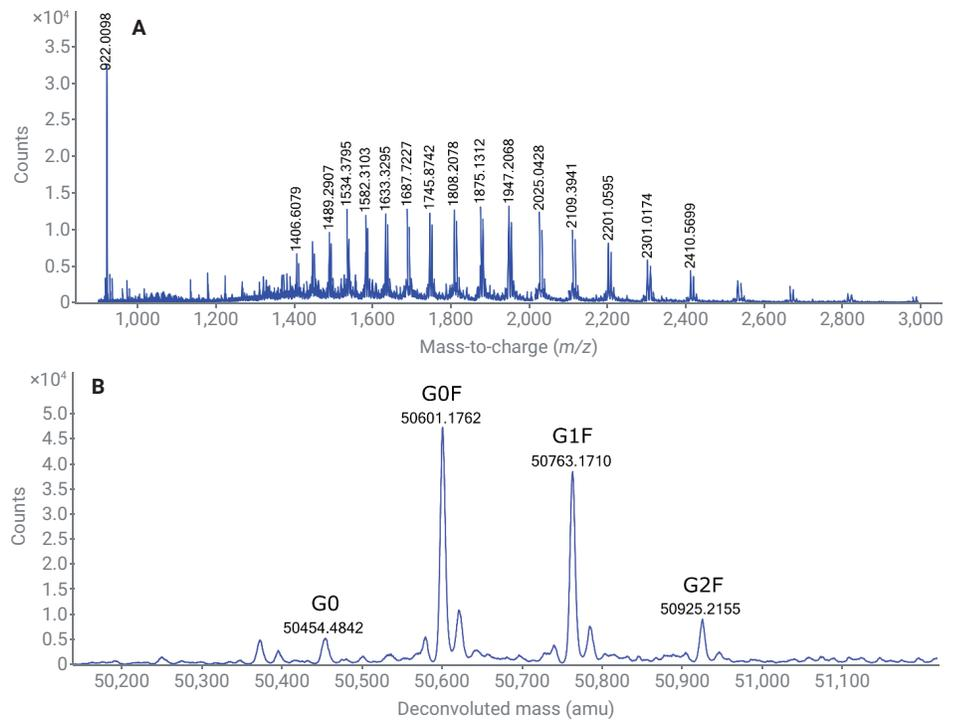
**Figure 4.** Extracted mass spectrum (A) and deconvoluted mass spectrum (B) of the heavy chain of Trastuzumab.
