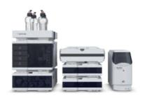
The InfinityLab HDR-DAD Impurity Analyzer quantifies sample components with widely different concentrations in a single assay.
