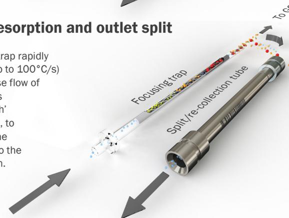
During either stage, the flow of analytes can be split and re-collected onto a clean sorbent tube.
