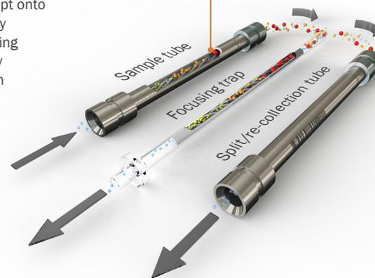
Sample tubes and traps can contain multiple sorbents, for analysis of an extended range of analytes.
