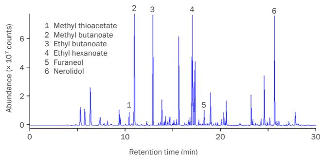
**Aroma-profiling foods and beverages** is widely studied using TD. In this example, Markes' Micro-Chamber/Thermal Extractor is used to quickly profile a range of aroma compounds from strawberries in a single run.
