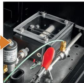
The trap is thermally desorbed at up to 100°C/s to inject the sample into the GC-MS as a narrow band.
