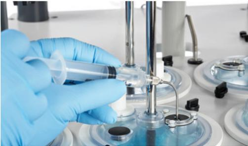
Increased method storage and easy sampling through evaporation covers make manual sampling easy with the 708-DS.
