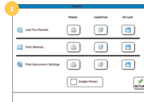
Various options exist for exporting data from the 850-DS including printer, serial port (RS232), or SD card.
