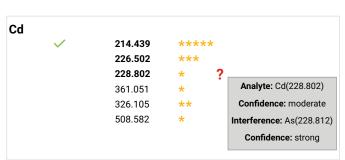
IntelliQuant Star ranking output for Cd. A five-star ranking with green check mark indicates Cd 214 wavelength to be the best. The red question mark indicates there is an issue on Cd 228, and the pop-up tip indicates the Cd 228 result has only moderate confidence as it has a strong arsenic interference.
