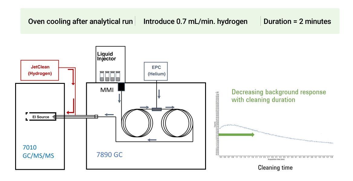
Instrument schematic (left). JetClean is a patented option that adds a controlled flow of hydrogen directly into the ion source to provide a cleaning action. The cleaning process occurs when the filaments are on and only affects the source. Cleaning can be done during the analysis (Acquire and Clean mode) or as a separate method following the analytical run (Clean Only mode). The latter case may take advantage of the fact that the oven is cooling during this time.
