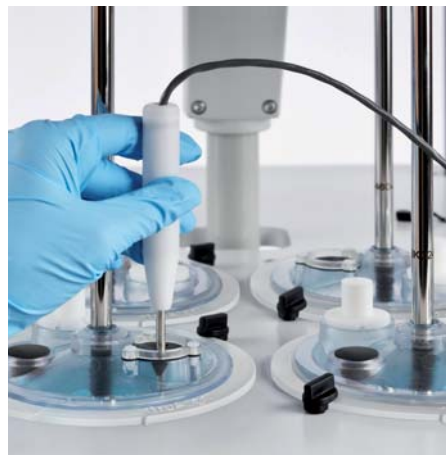
Manual temperature measurement using 708-DS integrated hand-held temperature probe.
