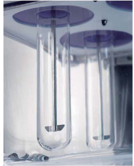
The 200 mL EaseAlign conversion kit (p/n 12-0318) contains a vessel adapter, mini-paddle, and 200 mL vessel for small volume dissolution testing.
