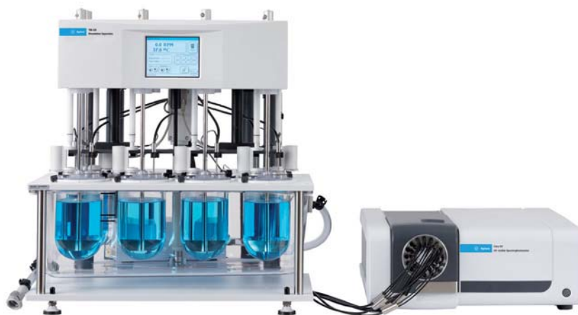
708-DS Dissolution Apparatus and Cary 60 Fiber Optic UV Dissolution system.
