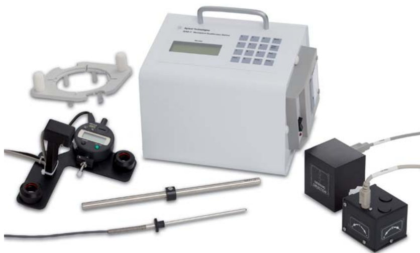
QAll C Mechanical Qualification Station.
