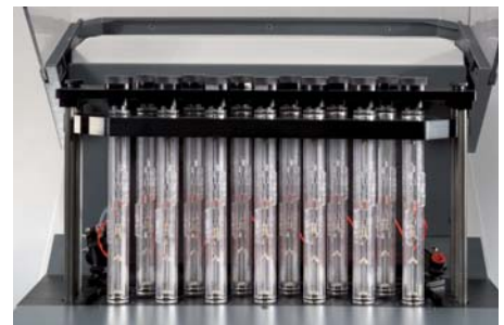
Internal view of cell holders.
