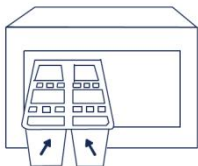
Figure 8-15: Slide the new reagent cartridge into the reagent compartment
