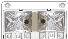
Figure 7-15: Seal the loading wells of FCS SE100 cartridge
