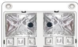
Figure 7-8: Pierce the seal of FCL PE100 or FCL PE150 cartridge
