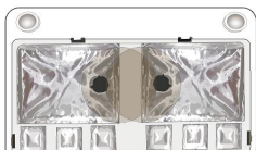
Figure 7-7: Seal the loading wells of PE100 cartridge
