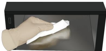
Figure 8-15: Maintain the reagent compartment
