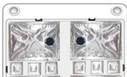
Figure 7-6: Pierce the seal of PE100 cartridge
