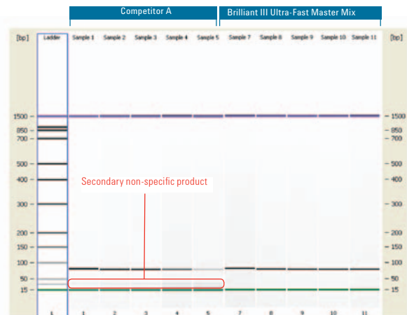
Figure 4. Trace of TBP qPCR products generated using Competitor A (left) or Brilliant III Ultra-Fast Master Mix (right) run on Agilent 2100 Bioanalyzer. Presence of primer-dimers/non specific amplification is evident when Competitor A master mix is used for amplification.
