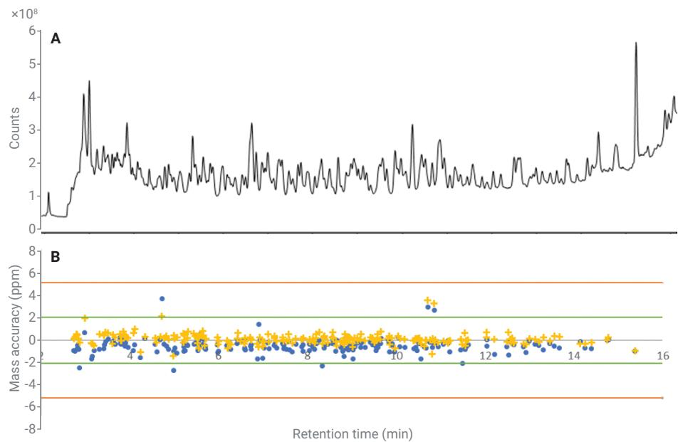
**Figure 5.** Total ion current (TIC) of a strawberry sample (A) and the mass accuracy of priority target ions in strawberry matrix at 10 ppb (blue circles) and 100 ppb (yellow crosses) plotted against their RT (B).
