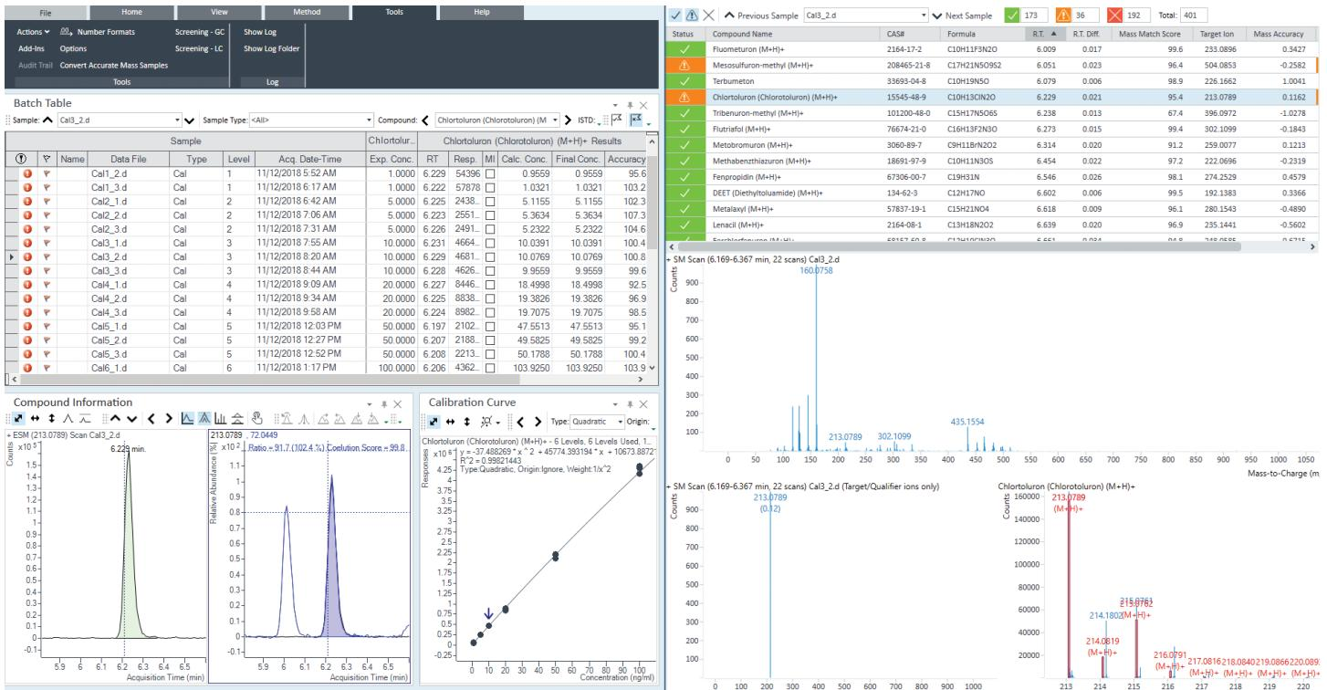
**Figure 3.** LC/Q-TOF Screener tool displayed next to the classic UI. Selected in the Screener results is a compound that has a calibration curve in the analysis. This analyte would be considered a priority target, and can be quantitated.
