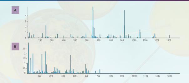
Agilent All Ions MS/MS is used to identify low-level peptides in a complex serum mixture. The starred peak in the LC separation had 6 to 7 peptide components seen separated in drift time heat map above. These could not be detected and identified using just LC and MS. A) Sum of fragment ion spectrum at 30 V across the starred peak. B) Drift separated fragment ion spectrum of the triple charged HLVDEPONLIK peptide at 20.26 ms.
