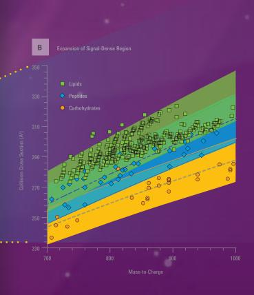
B) is a zoomed-in region where a high density of signal occurs. Distinguishing individual ion signals by the m/z measurement alone is challenging, yet the combined structural separation of IM Q-TOF provides a means of delineating the data into chemical class-specific regions.\*
