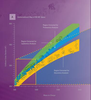
A) Complex sample containing a mixture of lipids, peptides, and carbohydrates was infused directly into the instrument and resolved in 2-D IM Q-TOF analysis by collision cross-section and m/z. Conformational space maps allow complex mixtures to be separated based on different biomolecular
