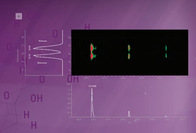
Separation of isobaric trisaccharides using IM Q-TOF: A one-to-one mixture of melezitose and raffinose was infused using a syringe pump. These two carbohydrates can be baseline separated using the ion mobility drift cell and detected using the Q-TOF mass analyzer as sodium adducts. The ion mobility resolving power for this separation is 60.
