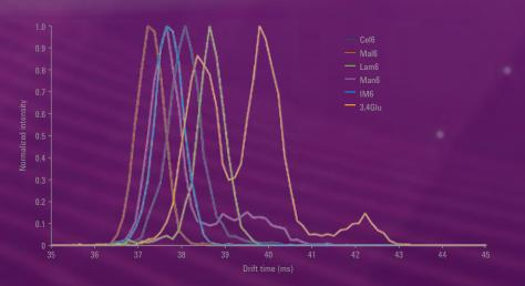
IM Q-TOF separation of permethylated oligosaccharides. These oligosaccharide samples were infused separately and analyzed using IM Q-TOF as sodium adducts. These isobaric hexoses show different drift distributions, indicating their structural differences. Ion mobility separation is a valuable technique that can be used to separate isobaric compounds with different structures.
