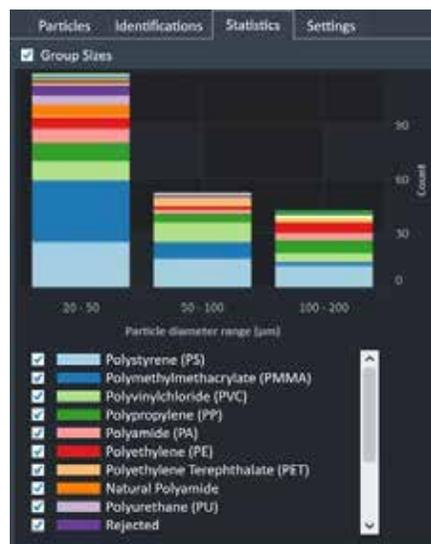
The 8700 LDIR will report what percentage of the total number of microplastic particles each type of plastic represents (top). It will also report a range of statistics, like the number of particles of each plastic type that fall into different particle size ranges (bottom).
