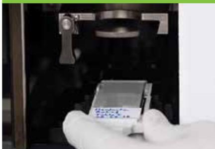
**Step 3.** The instrument will scan an area using light of a single wavenumber to locate all the particles. It takes only 4 minutes to scan an area 10 x 10 mm at 5 µm pixel size. The instrument then targets the identified particles (appearing as bright spots) and collects an IR spectrum of each one.
