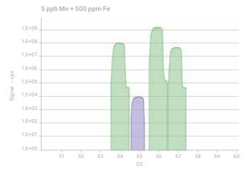
Figure 2. He MS/MS mode spectra: (top to bottm) 5 ppb Mn, 500 ppm Fe, and 5 ppb Mn + 500 ppm Fe.
