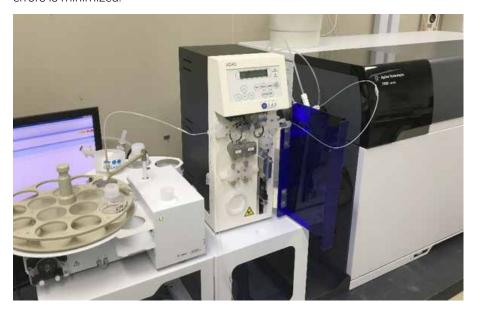
**Figure 1.** An Agilent ICP-MS fitted with an IAS ASAS automated standard addition system and the Agilent I-AS integrated autosampler.
