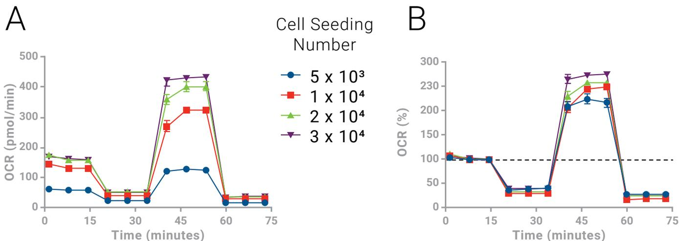
**Figure 4.** Absolute vs. Baselined OCR data: Panel A shows absolute OCR with a correlation of respiration rate to cell number. Panel B shows that for each cell density, responses to XF Cell Stress Test compounds are approximately equivalent, however information regarding differences in OCR with respect to seeding density is lost upon transformation with the Baseline feature.
